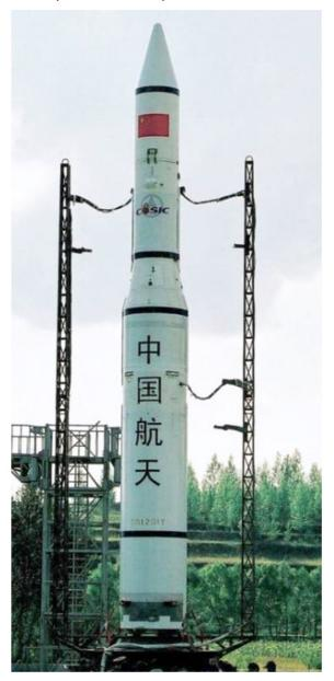
Kaituozhe-1 (KT-1) was small, solid fueled launch vehicle based on the road mobile DF-21 IRBM with an additional upper stage (in total 4 stages). It was 13.6 meters in length and 1.4 meters in diameter, with launch mass of 20t. It was possible to launch KT-1 both from a truck-based platform or from airborne platform. It had a 100 kg to LEO payload capacity. It was possibly the launch vehicle for a Chinese ASAT system that was tested against an old Chinese weather satellite in 2007.
